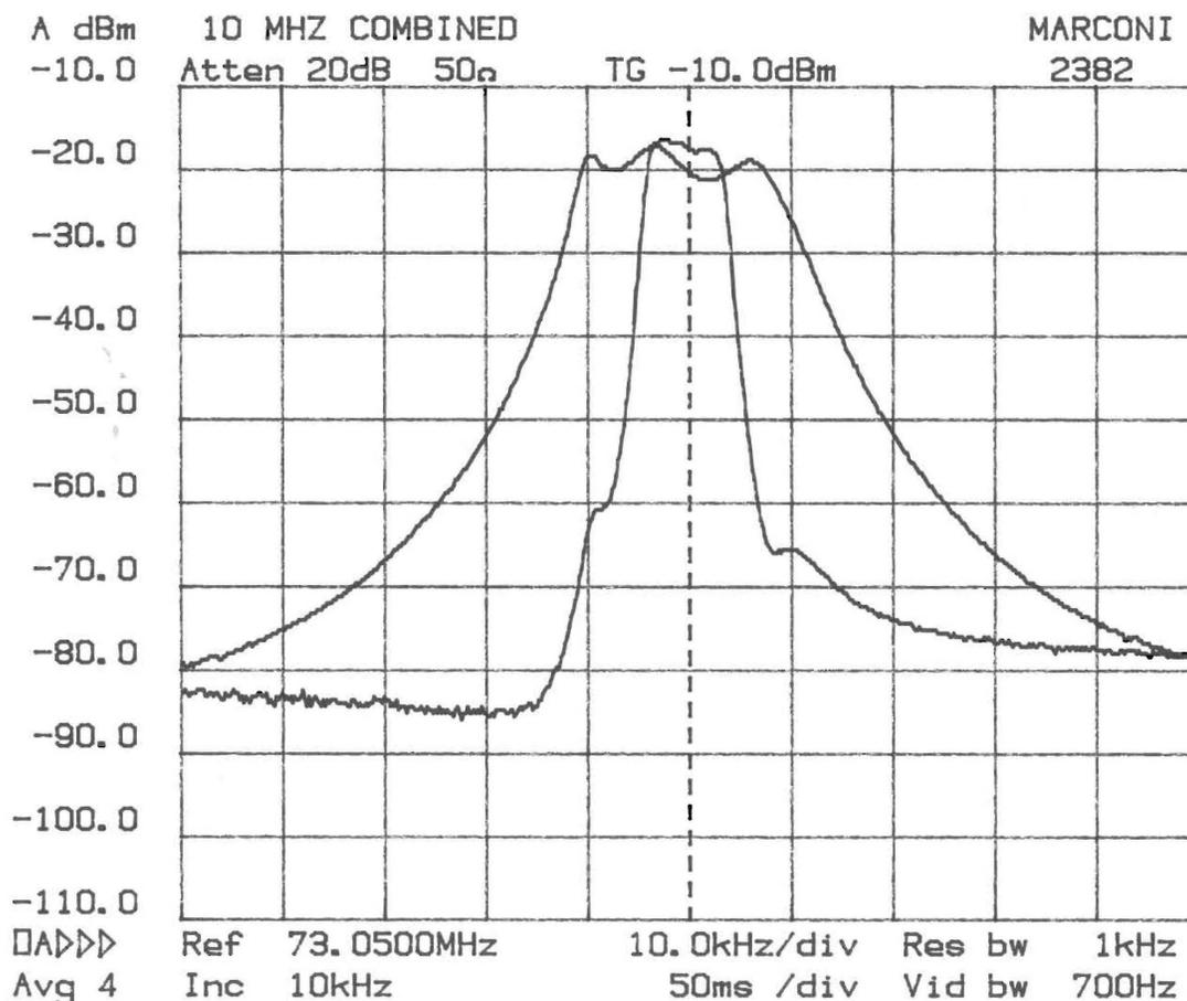
The result of the bandwidth improvement is the reduction of close in intermodulation from multiple signals. The IMD dynamic range will be improved up to 15 or more dB for signal spacings from 2 to 20 kHz. Also, the blocking dynamic range will be improved for close in signals.
